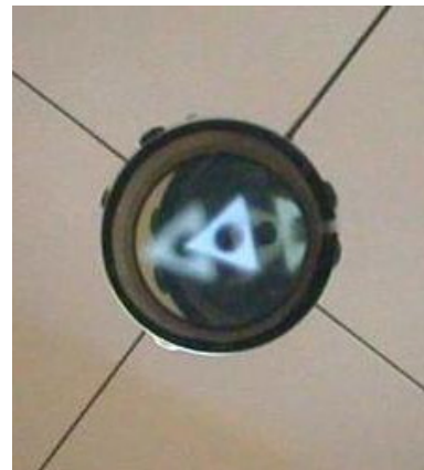
Autocollimator image of residual misalignment (Secondary tilt & rotation)
